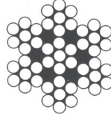
NIRO-Drahtseil NIRO Wire rope 6 x 19M-WSC
